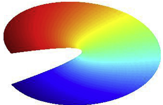
Fig. 5. Crack face displacement discontinuity reproduced by the crack tip enrichment function \sqrt{r}\sin(\theta/2) .
