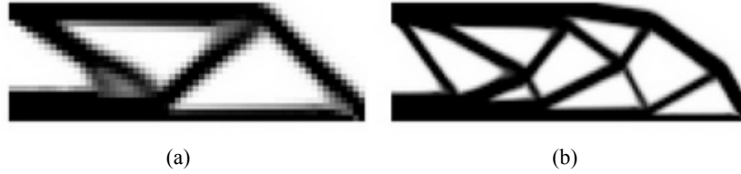
Figure 8. Mesh-dependency - optimum topologies of MMB problem using 60x20 (a) and 120x40 (b) mesh sizes
