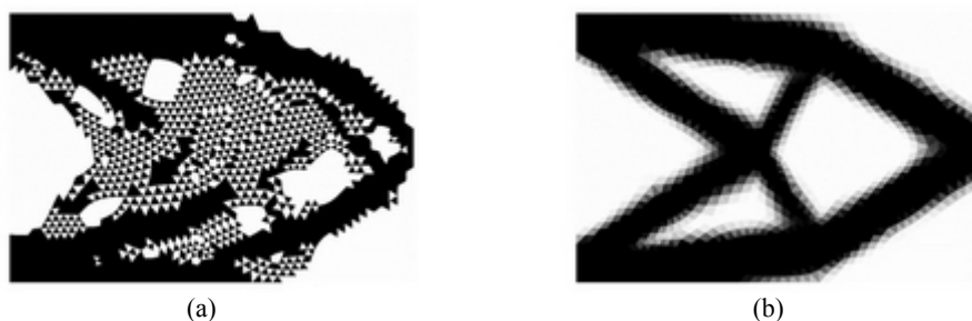
Figure 6. Using unstructured mesh of CST elements - optimum topologies obtained by normal SIMP method (a) and by the new approach (b)
