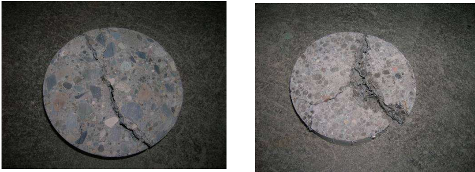
FIGURE 2 - FAILURE PATTERNS OF SPECIMENS
