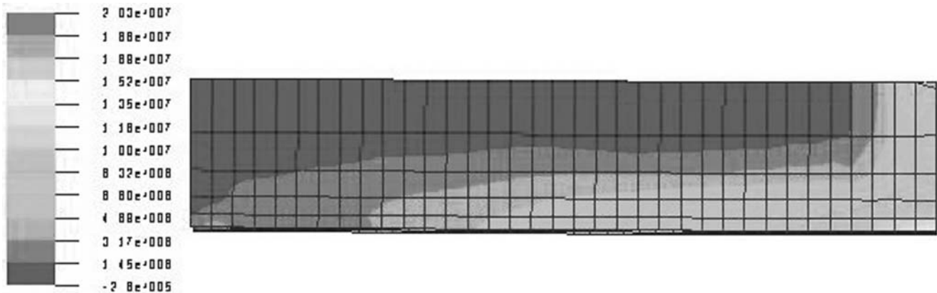
Figure 12. Contour of maximum principle stress in Pa at time step=.00075 s
