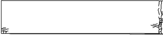
Figure 17. Cracking Pattern at time step=.000165s
