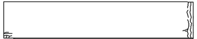
Figure 15. Cracking Pattern at time step=0.00075s
