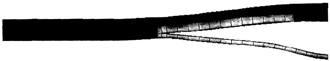
Fig.13: Final global buckling
