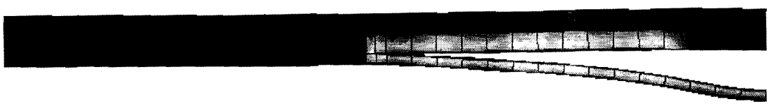
Fig.12: Commencing of global buckling
