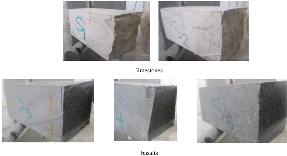
Fig.5: Fractured surfaces of limestones and basalts specimens under dynamic loading
